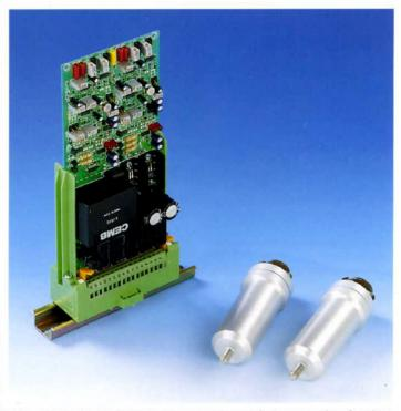
The processing module, which can be fitted on a DIN guide EN 50022 inside a control panel, features a series of settings which can be made by the customer for selecting optimum measuring parameters, delay time for the alarms, scale range, etc. The module is implemented with SMD technology to compact size and improve reliability.
